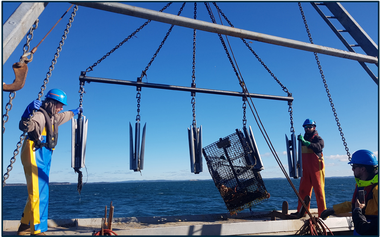
Towed grapnel system with recovered shellfish trap. CSR GeoSurveys Ltd.
