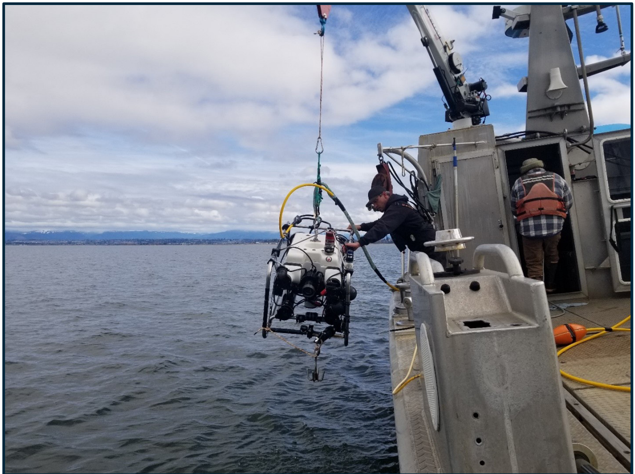
Working class ROV fitted with grapnel being deployed to retrieve Dungeness crab pots from waters below diver depth. NRC
