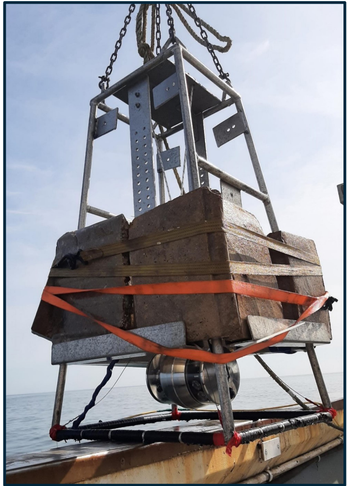
Deep Trekker DTPod camera on custom fabricated steel frame with concrete weights Comité ZIP des Îles
