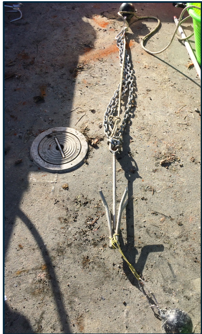
Single grapnel designed to catch ropes and weighted to maintain depth and position. Used to retrieve Dungeness crab traps after trap locations were identified using sidescan sonar. NRC
